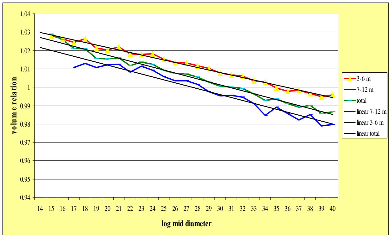
Fig. 10. The relationship between the volume of logs determined according to the ČSN 48 0050 Standard – Rough timber – manual measurement and a comparative method. The dependence of the relationship on the log mid diameter (x axis) and the length of logs (logs 3-6 m and logs 7-12 m). The total dependence (not distinguishing lengths) is expressed as a green line.
