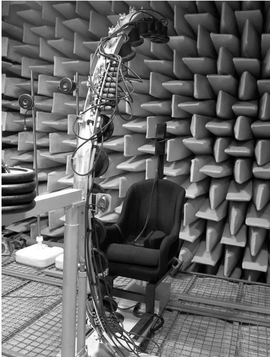
Fig. 1. Overview of the HRTF measurement equipment.
