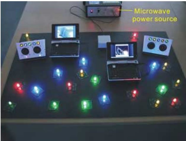
Fig. 12. Power supply via the communication sheet to small devices including speakers, LED lights, monitors, etc.
