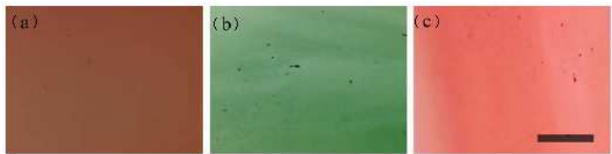
Fig. 17. Optical micrographs of drawn PVA-gold nanocomposites (4 % w/w gold, draw ratio 4): (a) unpolarized, polarization direction, (b) parallel and (c) perpendicular to the drawing direction. Scale bar is 50 mm (Park, 2006).
