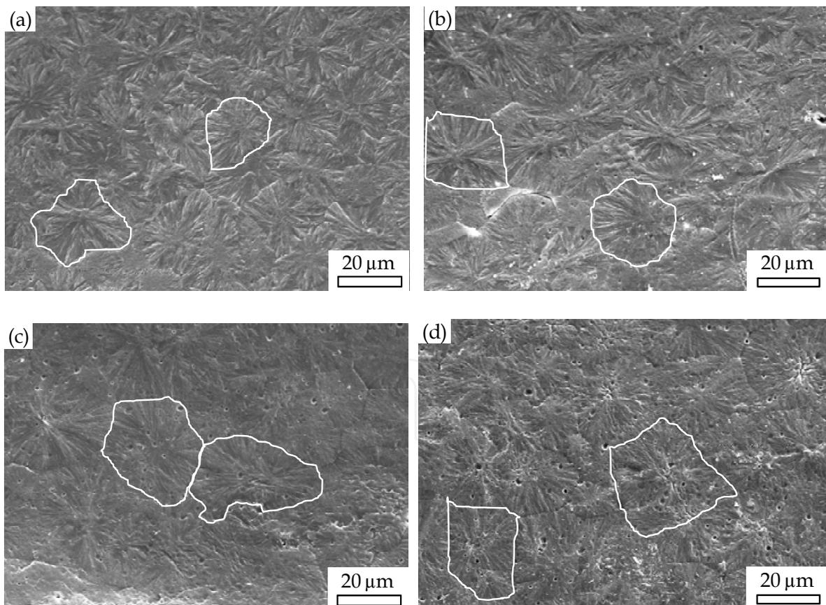
Fig. 1. SEM images at a magnification of  $\times 1000$  showing the spherulitic morphology of (a) polypropylene homopolymer, PP0, and controlled-rheology polypropylenes, CRPPs, with (b) 154, (c) 402 and (d) 546 ppm of peroxide content. By way of example some spherulites have been outlined with white lines.
