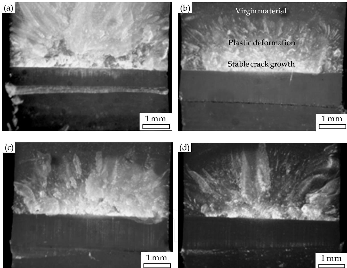
Fig. 6. Fracture surfaces obtained via light microscopy of (a) PP0, (b) PP-CR154, (c) PP-CR402 and (d) PP-CR546. All the specimens showed a stable crack length  $\sim 0.3$  mm. By way of example, the three characteristic regions appearing in the fracture surfaces are indicated in CRPP154 micrograph.
