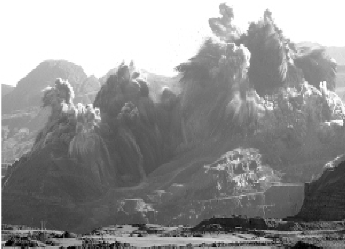
Fig. 7. Throw blasting in Dafeng mine.
