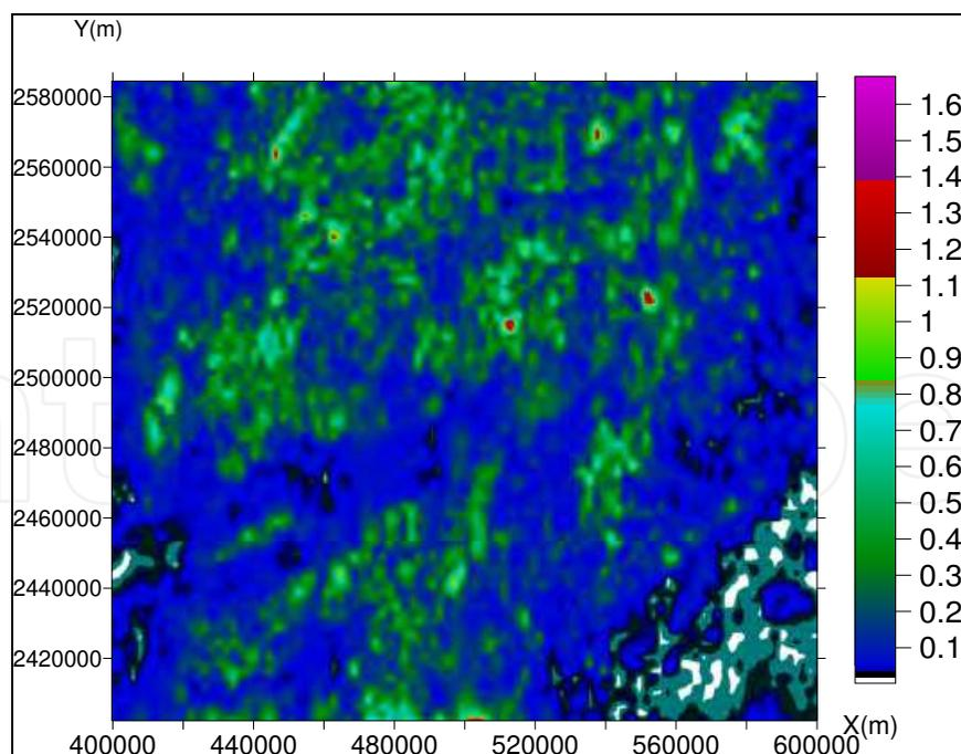
Fig. 12. Amplitude of the analytic signal of the anomaly magnetic field of In-Ouzzal
