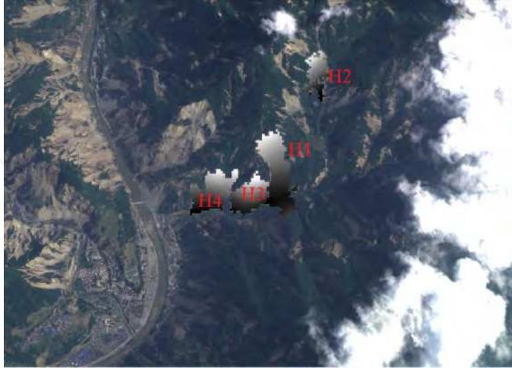
Fig. 27. Identified landslides as loose material of the debris flow
