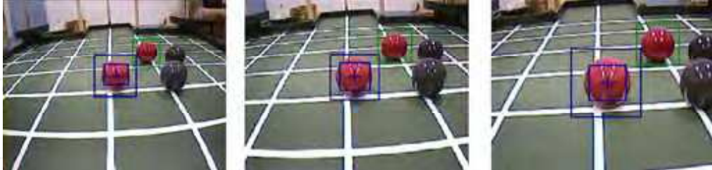
Figure 7. 3-D tracking of red balls. A camera is mounted on a wheeled robot which is moving in the ground plane (basketball robot players). Given the radius, red balls should be tracked and picked up
