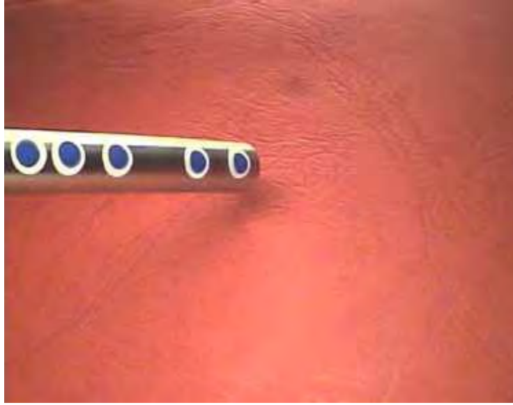
Figure 4. Collinear points (centroids of blue markers) stuck on a metallic and cylindrical surface
