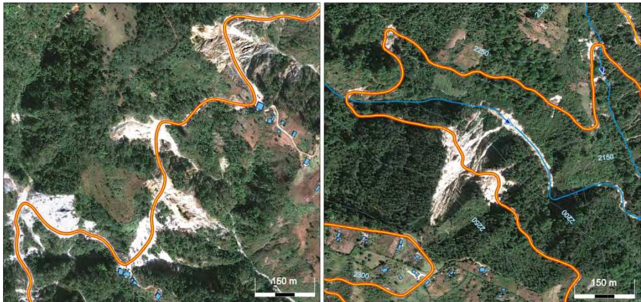
Fig. 16. Roadside slides above Buenos Aires (left; locality Las Flores Buenavista, road towards Porvenir) and below Niquivil (right; locality Tuxchamén, dirt road towards Pavencul). Blue quadrates = houses and sheds, blue line = creek with arrow of flow, red-yellow lines = roads (source Google maps, date taken November 2010)
