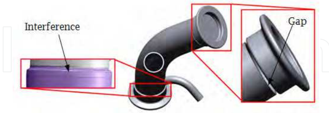
Fig. 20. Gap and interference between solid features in the tubing model
