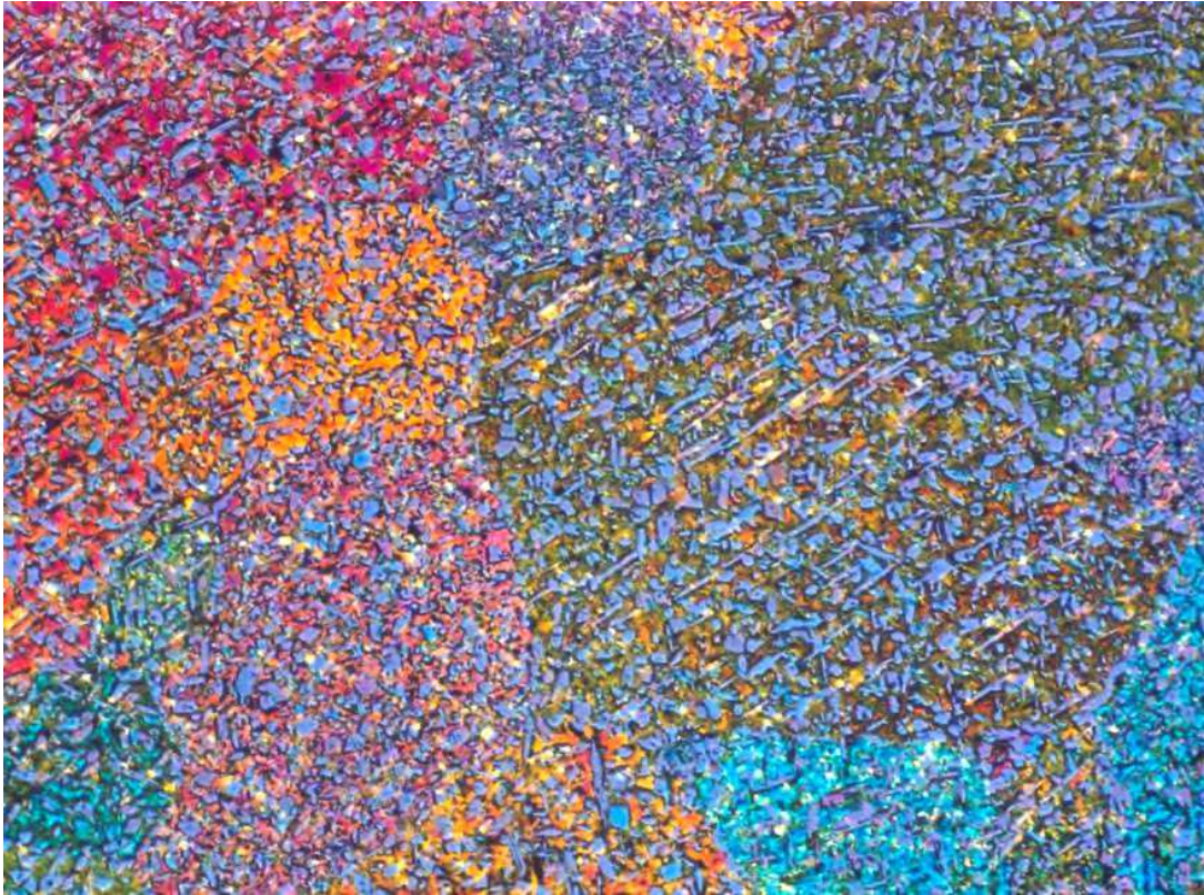
a) polyhedral microstructure, mag. 100 x
