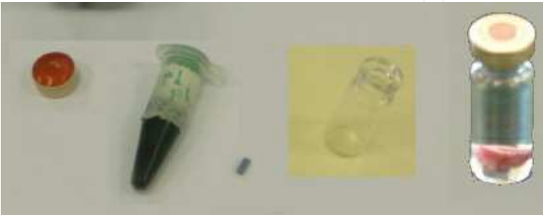
Fig. 2. A sealed reaction vial containing Pd phosphor solution, stirring bar and a mouse liver specimen.
