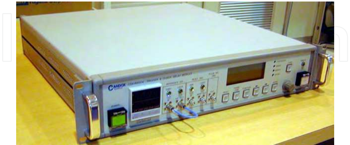
Fig. 6. High precision RF phase control circuit. The circuit provides a delayed RF signal from the output port with a precision of better than 3 ps (in rms) which is independent of the delay time.
