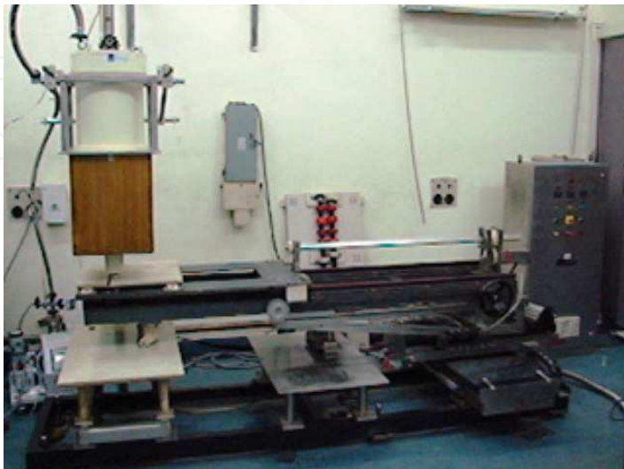
Fig. 8. Photograph of the SQUID based NDE system
