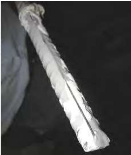
Fig. 19. Interlocking surface in an anchor installed into a hole which is not filled with epoxy (Photo by Dr. Halil Nohutcu)
