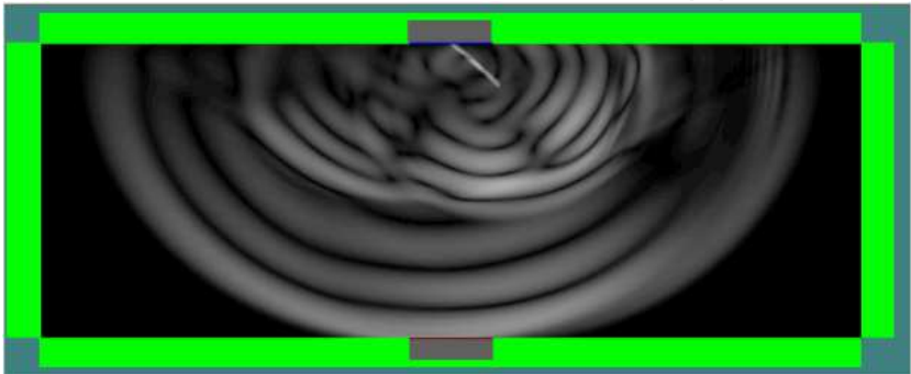
Fig. 2. Acoustic Emission Wave Propagation in fractured Material
