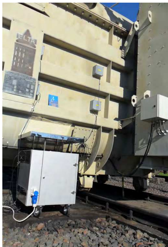
Fig. 1. System for large power transformer on-line monitoring based on AE method
