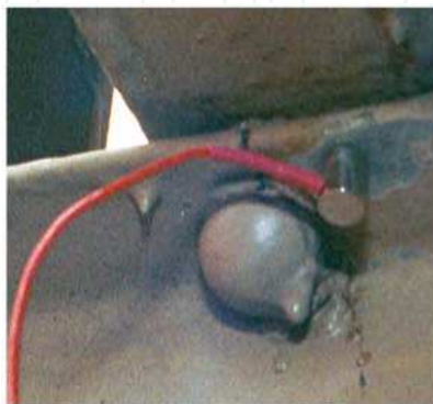
Fig. 2. AE Sensor on Brooklyn Bridge Floor Beam
