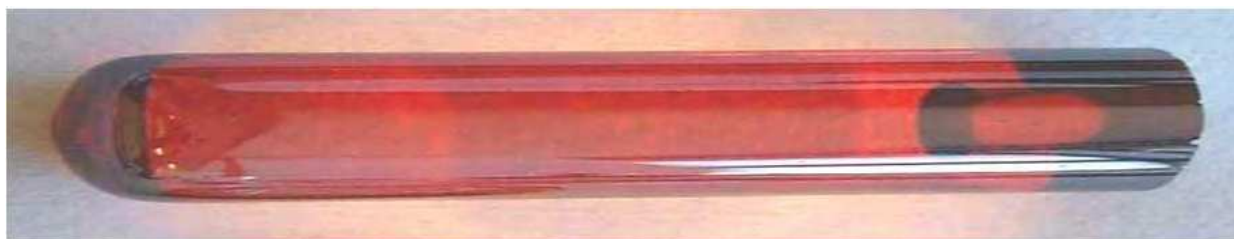
Fig. 2. Example of glass rod of the \text{GeS}_2\text{-Sb}_2\text{S}_3\text{-CsCl} composition.
