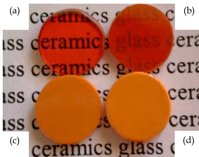
Fig. 5. Glass composition 62.5\text{GeS}_2\text{-}12.5\text{Sb}_2\text{S}_3\text{-}25\text{CsCl} heated at 290^\circ\text{C} for different crystallization times (a) No thermal treatment (b) 7h (c) 73h and (d) 144h.
