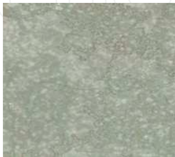
a. casting with no porosity
