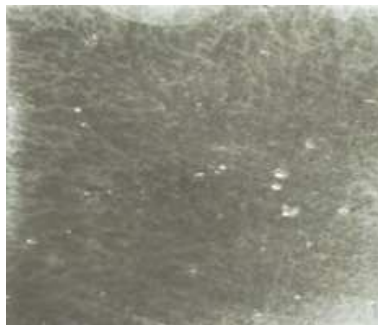
b. casting with classified porosity
