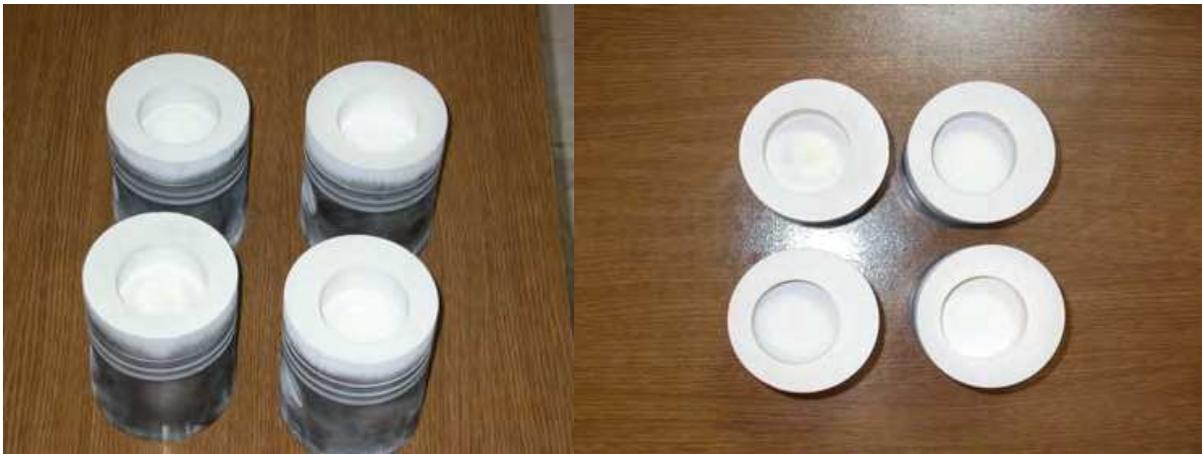
Fig. 10. Ceramic coated piston tops
