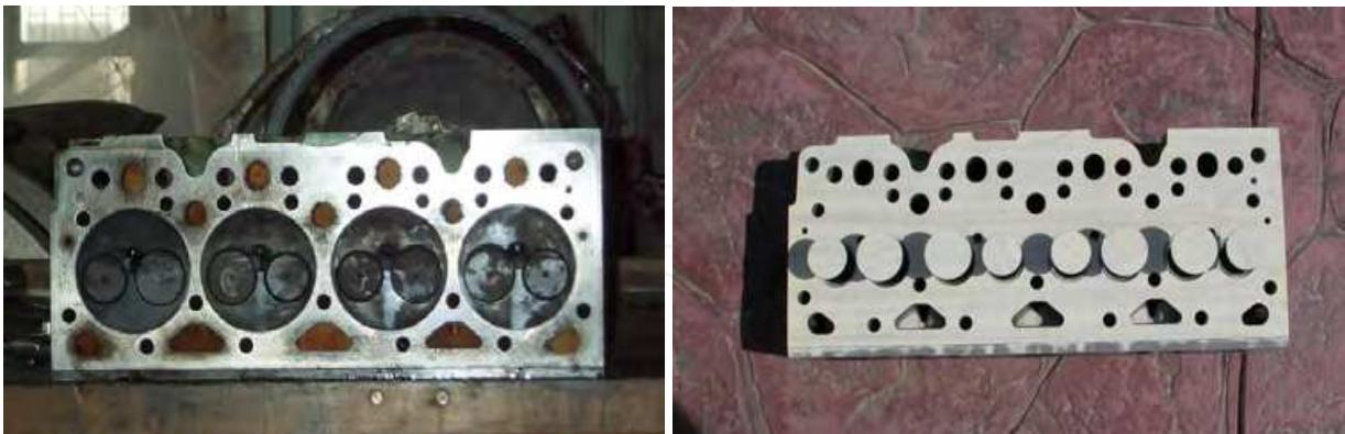
a) Cylinder heads and valves without coating b) Ceramic coated cylinder heads and valves
