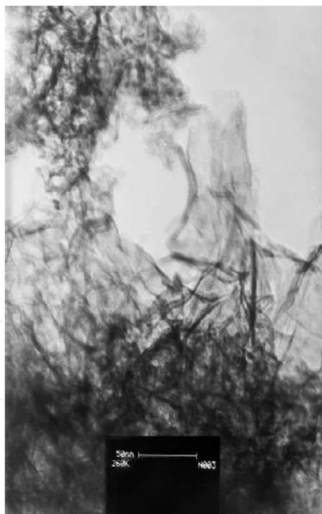
Fig. 14. Scanning electron microscope (SEM) (a) and transmission electron microscopy (TEM) (b,c) images of amorphous calcium - manganese oxides. These readily synthesized manganese-calcium oxides are the closest structural and functional analogs to the native the WOC of PSII found so far.
