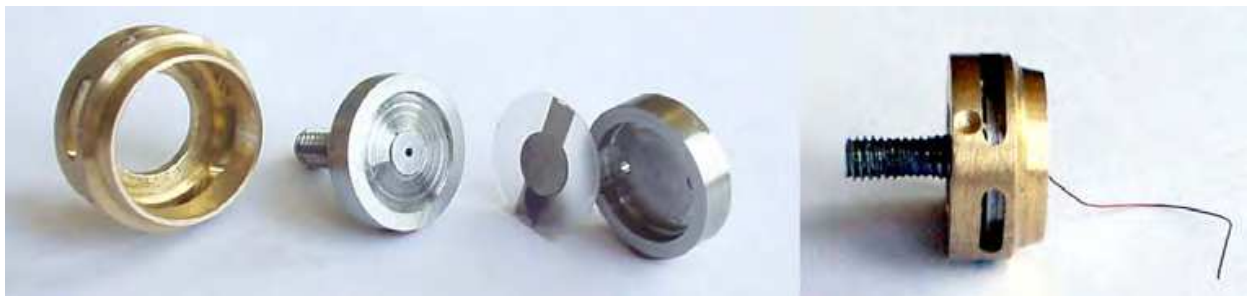
Fig. 22. Elements and construction of PRMT with PM
