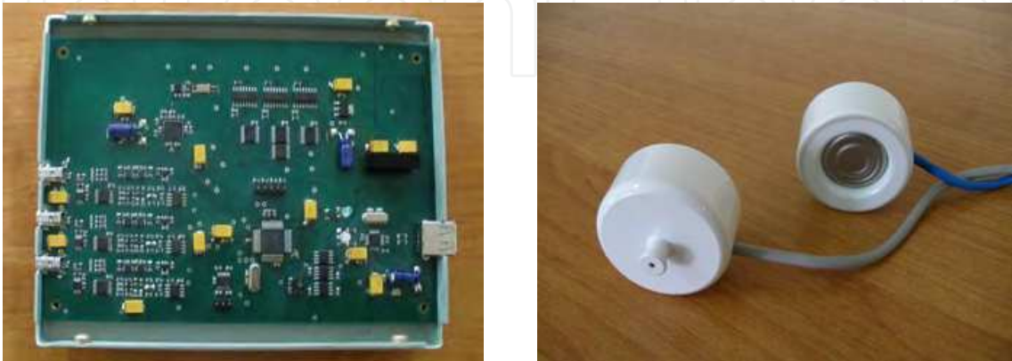
Fig. 27. Constructive realization of the block of the microcontroller and sensor of surplus pressure on the basis of PRMT
