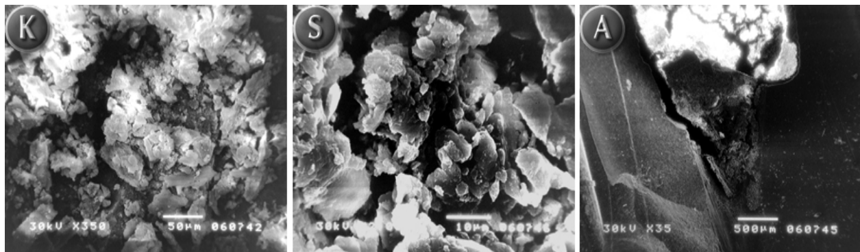
Fig. 5. SEM micrographs of coronal (K), middle (S) and apical thirds(A) of the canal walls after engine driven treatment using NiTi files without irrigation. Massive accumulation of dentinal debris
