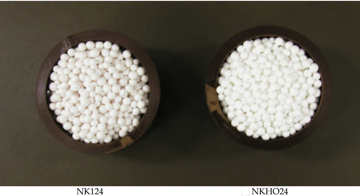
Fig. 2. Prepared alumina carrier-TiO 2 photocatalysts
