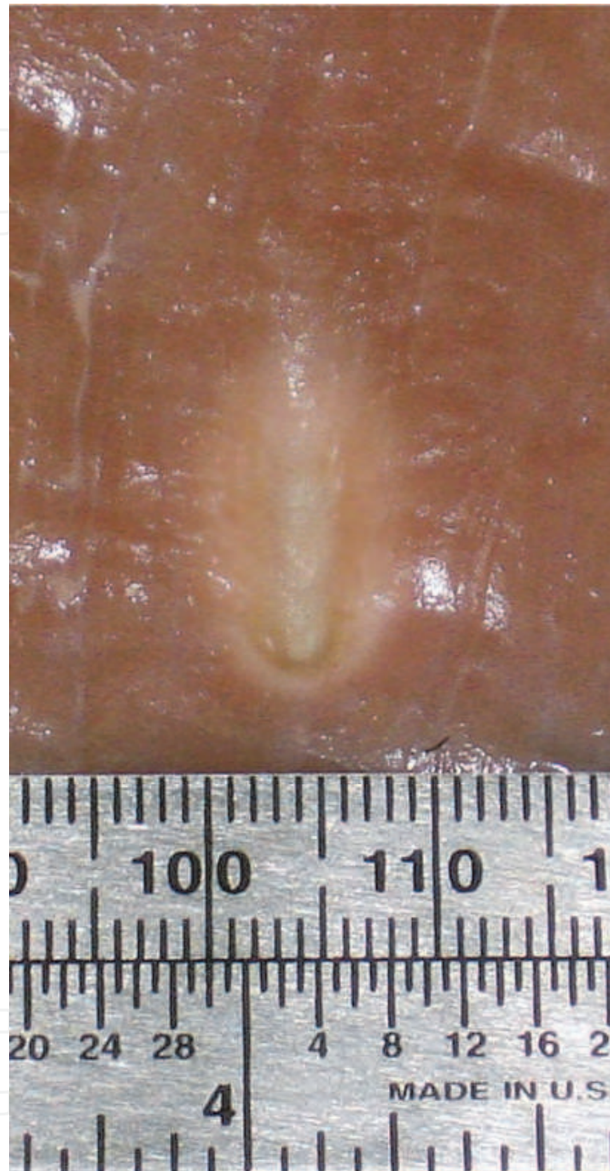
Fig. 9. A lesion created in an ex-vivo experiment at the end of a 180 s hyperthermia procedure.
