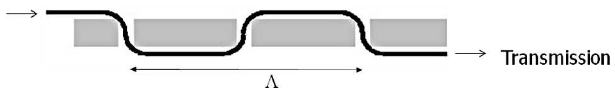
Fig. 10. Micro-bending of a multimode optical fiber
