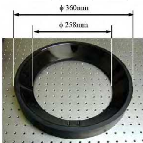
Fig. 75. Photo of aspherical mirror having off-axis paraboloid of revolution.
