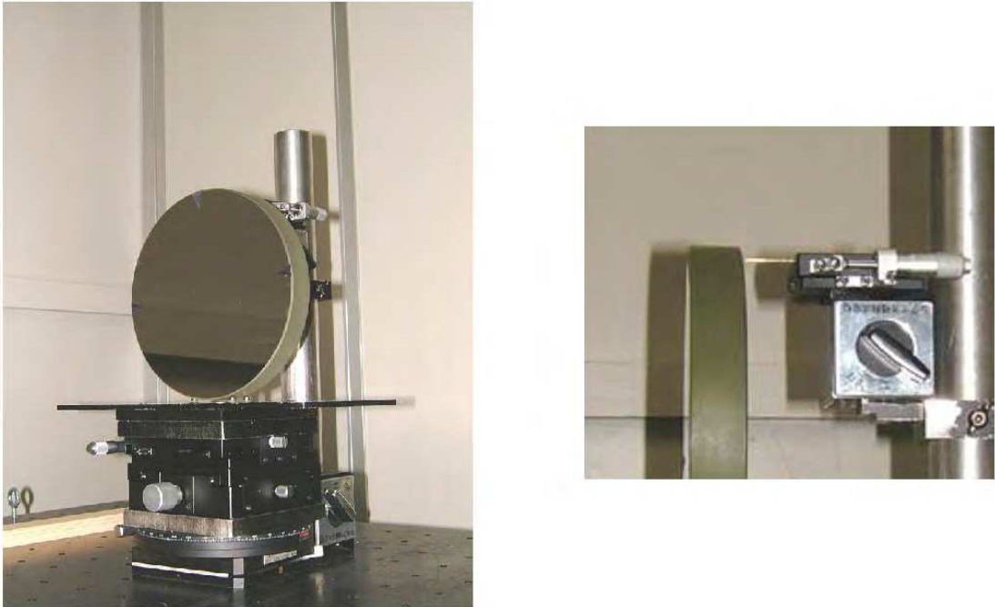
Fig. 51. Mirror supported by three-point suspension of steel balls and single needle.
