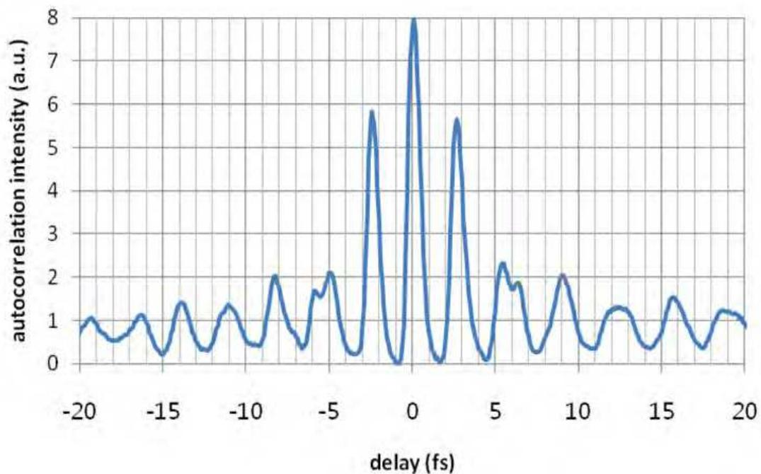
Fig. 9. (a) the measured pulse duration of 3.8 fs.
