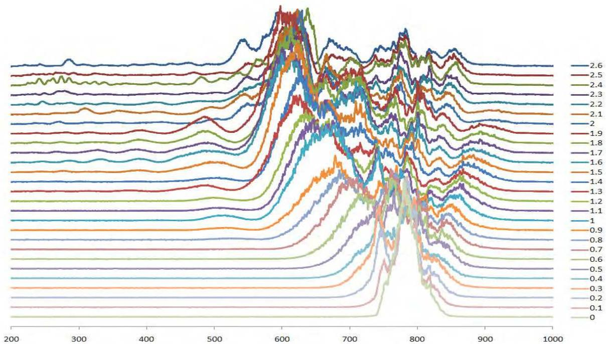
Fig. 8. Supercontinuum spectra vs Ne pressure (0 bar ~ 2.6 bar).
