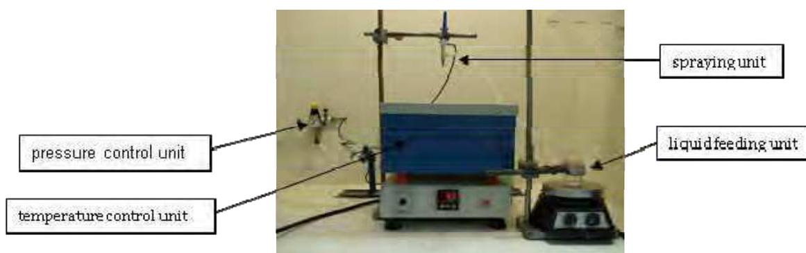
Fig. 3. Spray pyrolysis experimental apparatus.
