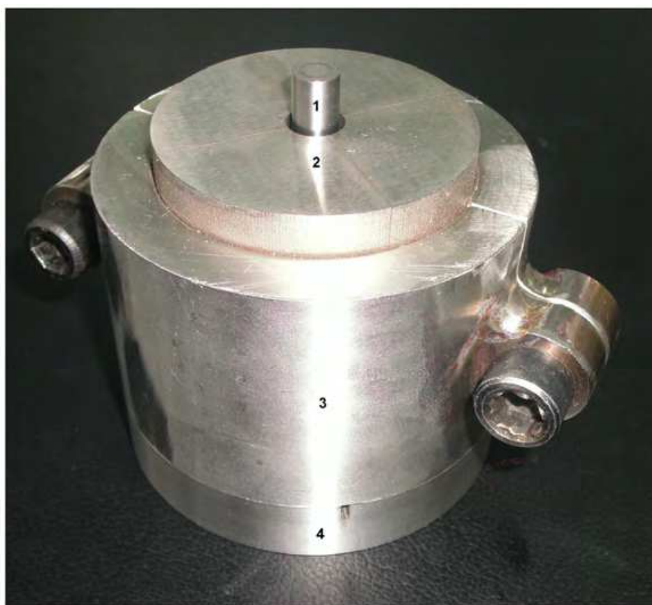
Fig. 2. The four-part dismountable mold is shown in this picture: 1-punch, 2-four-section dismountable block cylinder from high strength tempered steel, 3 - constricting clamp with two tightening bolts, 4 - support with groove for tungsten wire.
