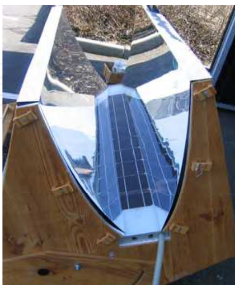
Fig. 1. Truncated CPC with 10 cell module string
