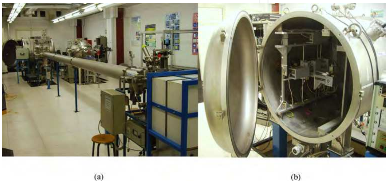
Fig. 7. (a) An overview of the LAX facility. (b) The detector chamber located at 10.5 m from the X-ray tube; the detection system was mounted on a XYZ microtranslator system.
