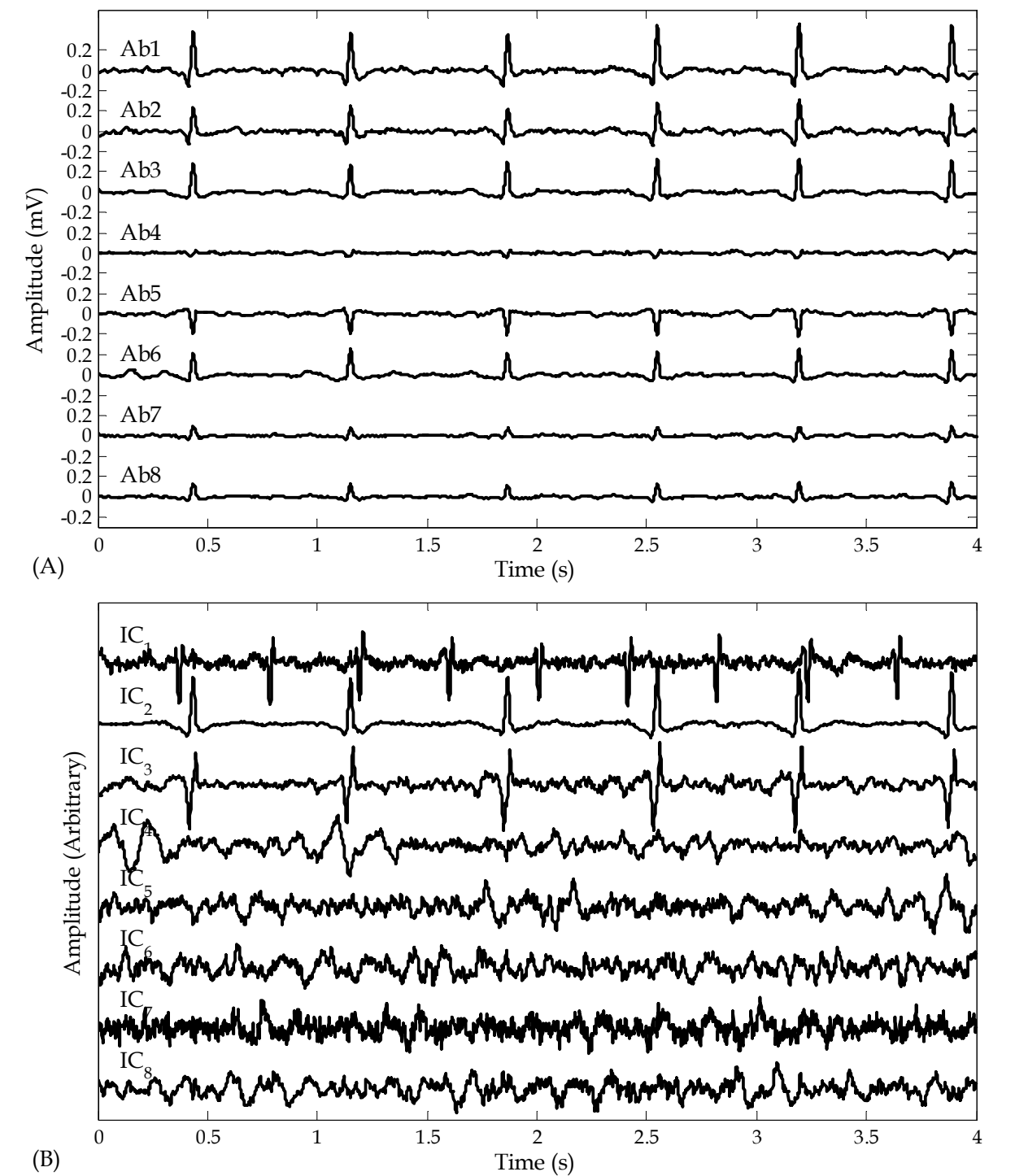
Fig. 4. (A) Eight-lead ECG measured on the abdominal region (leads Ab1 though Ab8) of a pregnant mother 1 . Maternal heart beats are clearly recognizable but fetal ECG cannot be visually observed. (B) Results of ICA on the data seen in (A). It can be clearly seen that IC 1 exhibits fetal ECG, whereas IC 2 and IC 3 carry maternal ECG.
