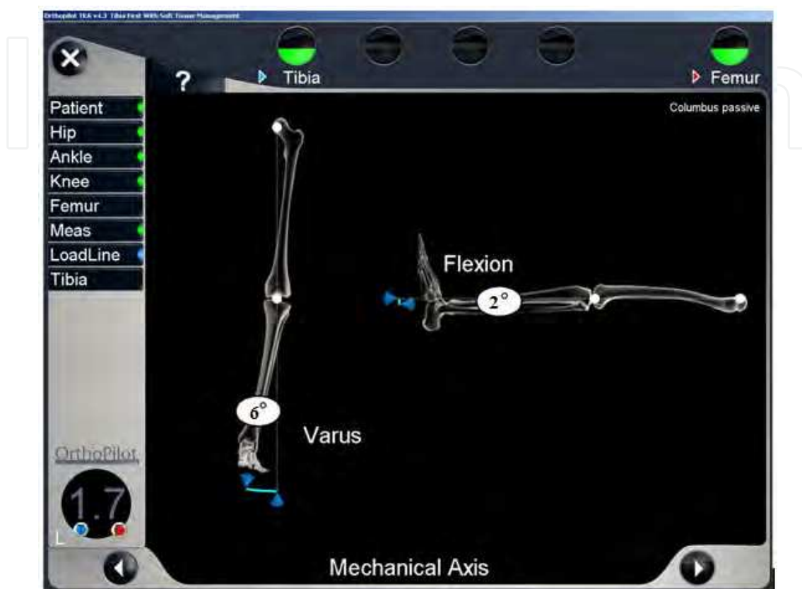
Fig. 6. The axis of the lower limb shown on the display of kinematic navigation system before UCA implantation
