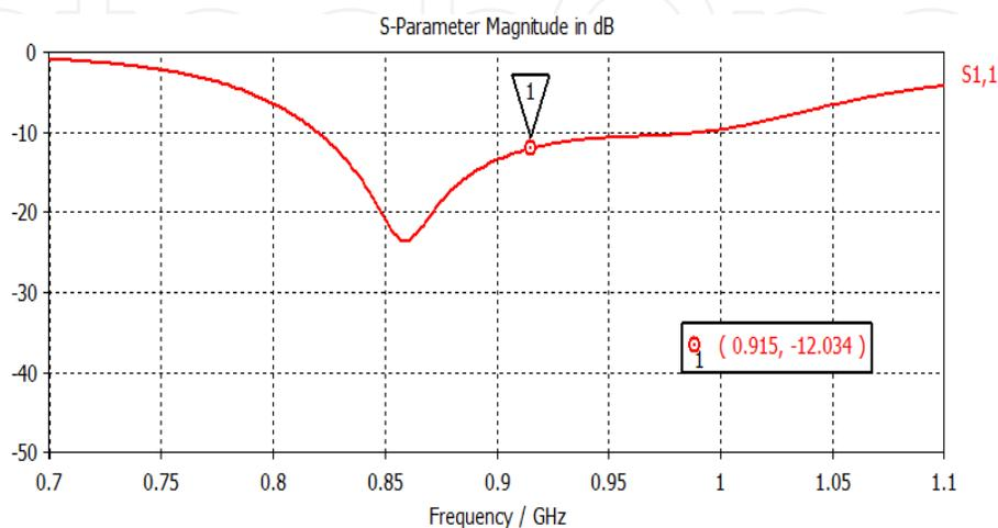
Fig. 16. Return loss of the metamaterial ZOR loop.
