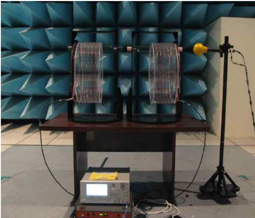
Fig. 3. WPT tested in a semi-anechoic chamber[2].
