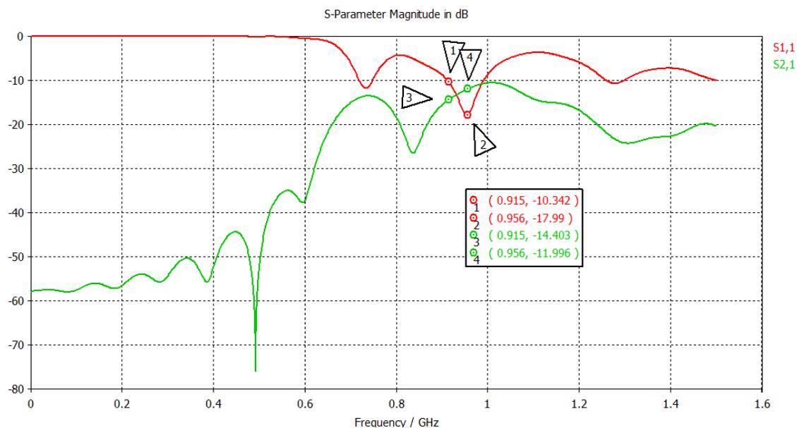
Fig. 21.  $S_{21}$  when the two MTM ZOR loops are 10cm away.
