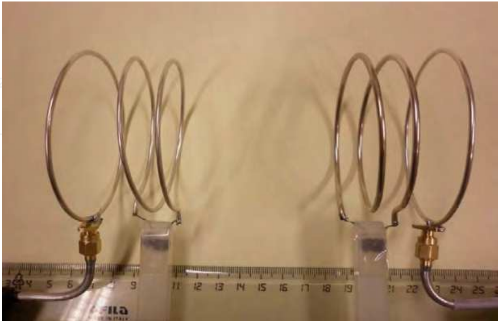
Fig. 2. A structure showing the inductive coupling between the source (first loop on the left), the transmitting resonator (second coil from the left), receiving resonator (third coil from the left) and load (last loop on the right).
