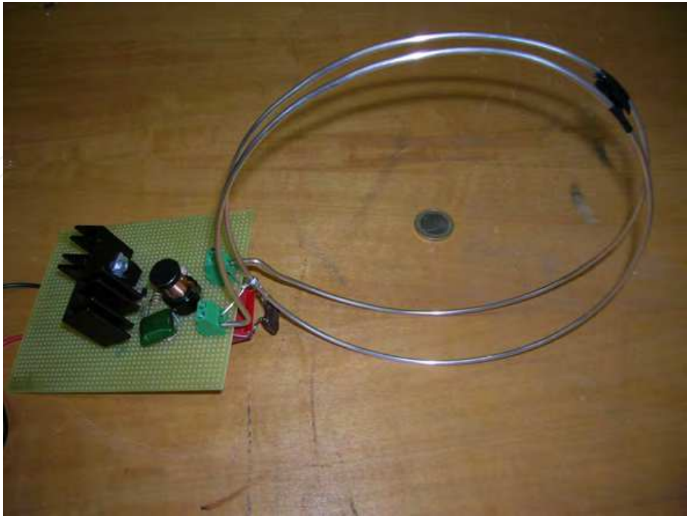
Fig. 25. Photograph of the transmitting circuit and the resonant conducting wire loops together with one euro coin. Note that the resonant coil is excited at its center.
