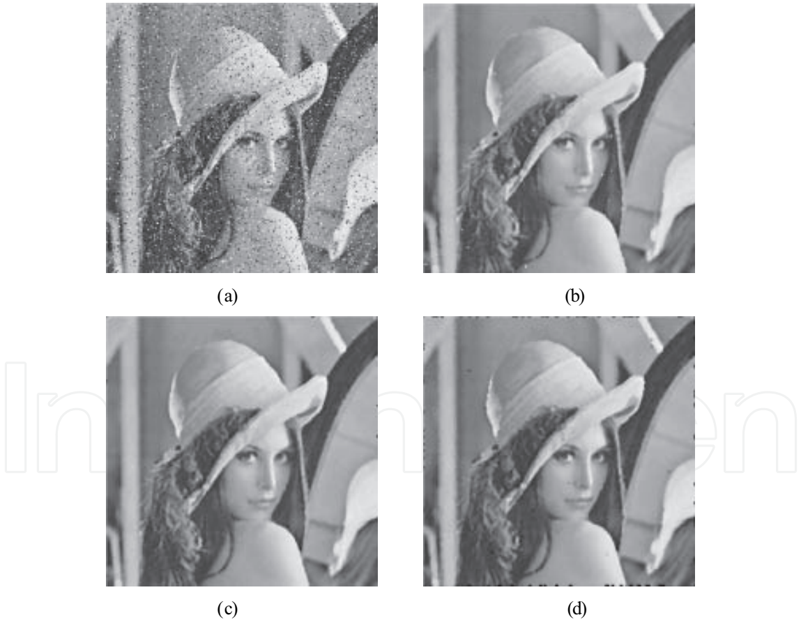
Fig. 41. Simulation results of a 2-D ROF application. (a) The noisy “Lena” image corrupted by 8% of impulsive noise. (b) The “Lena” image processed by the 3 \times 3 4th-order filtering. (c) The “Lena” image processed by the 3 \times 3 5th-order filtering. (d) The “Lena” image processed by the 3 \times 3 6th-order filtering.
