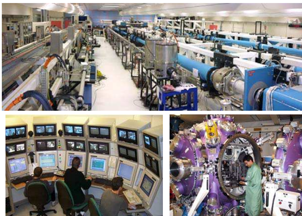
Fig. 1. LULI2000 laser facility: top: amplification chains; button left: command control room; button right: one of the interaction chambers "MILKA".
