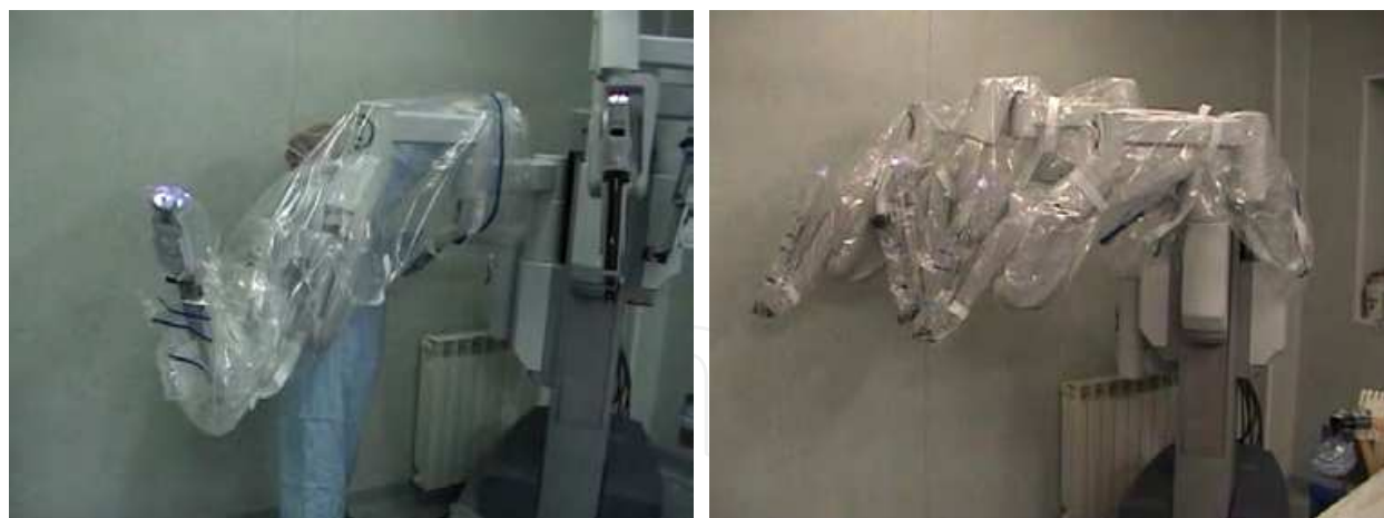
Fig. 5. Each instrument arm and the camera arm is draped separately
