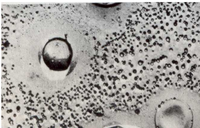
Fig. 9. Electron microscopic images of glasses (a) no. 1 and (b) no. 2 preliminarily heat treated at the temperature of 440 °C for 2 h and developed at 600 °C for 10 min.
