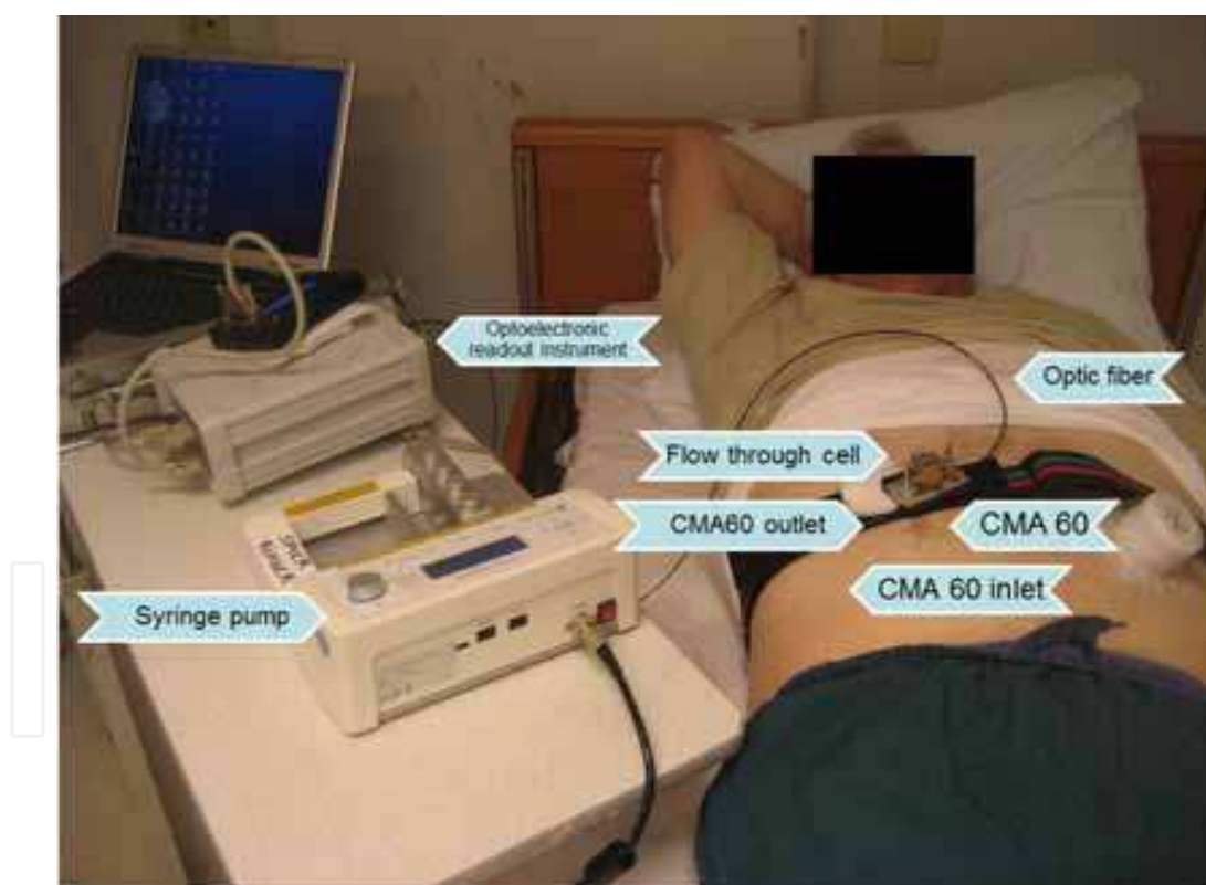
Fig. 4. Use of the optochemical oxygen sensor instrumentation during a typical in vivo experiment. The main components are the flow-through-cell, which is fixed near the umbilicus of the volunteer close to the position of insertion of the CMA 60 microdialysis catheter. The luminescence emitted by the oxygen sensitive membrane is collected by an optic fibre cable and guided to the optoelectronic read-out unit. The microdialysis probe is perfused using a microinfusion syringe pump. These experiments were carried out in the laboratory of Dr. G.H. Goossens (Maastricht University Medical Centre, The Netherlands).
