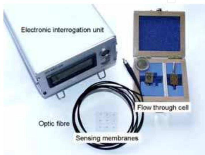
Fig. 2. Measurement system for planar sensing membranes. The flow-through cell has a size of 20 x 13 x 4.8 mm (length x width x height). The measuring chamber of the flow-through-cell has a diameter of circa 1.8 mm and a height of about 2.8 mm, thus resulting in a volume of about 5 \mu\text{l} . The sensing membranes have a round sensitive spot of 1.8 mm in diameter.
