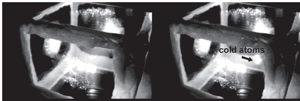
Fig. 26. Cloud of atoms obtained with surveillance camera. Left: no cloud, right: cloud of cold atoms.
