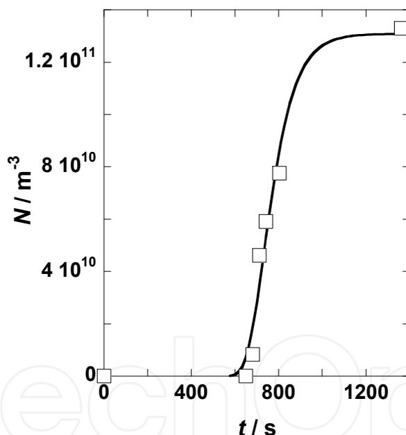
Fig. 3. Time course of the number of observed microcrystals at  $T = 20\text{ }^{\circ}\text{C}$ ,  $C = 27.07\text{ mgmL}^{-1}$ , and  $P = 100\text{ MPa}$  (Maruoka et al., 2010). Solid curve indicates a Gompertz function.
