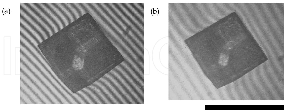
Fig. 1. Interferograms around the glucose isomerase crystal under 100 MPa (Suzuki et al., 2002b). Concentration of glucose isomerase in bulk solution is  $35.4 \text{ mgmL}^{-1}$ . (a) Growth ( $24.7 \text{ }^\circ\text{C}$ ), (b) dissolution ( $44.1 \text{ }^\circ\text{C}$ ). The scale bar represents 1 mm.
