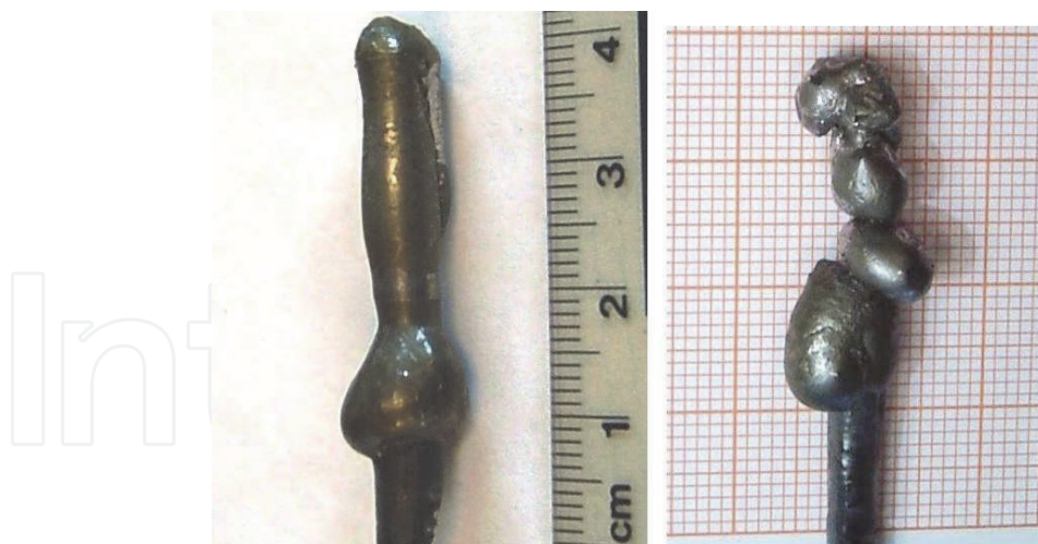
Fig. 2. Samples resulting from crystal growth experiments from the stoichiometric melt with upper and lower rod rotation. Left - Successfully grown single crystal ( sc1 ); Right - The crystallized ingot experienced repeated dropping down of the melt because of the unfavorable combination of the high density and of the low surface tension of the melt.
