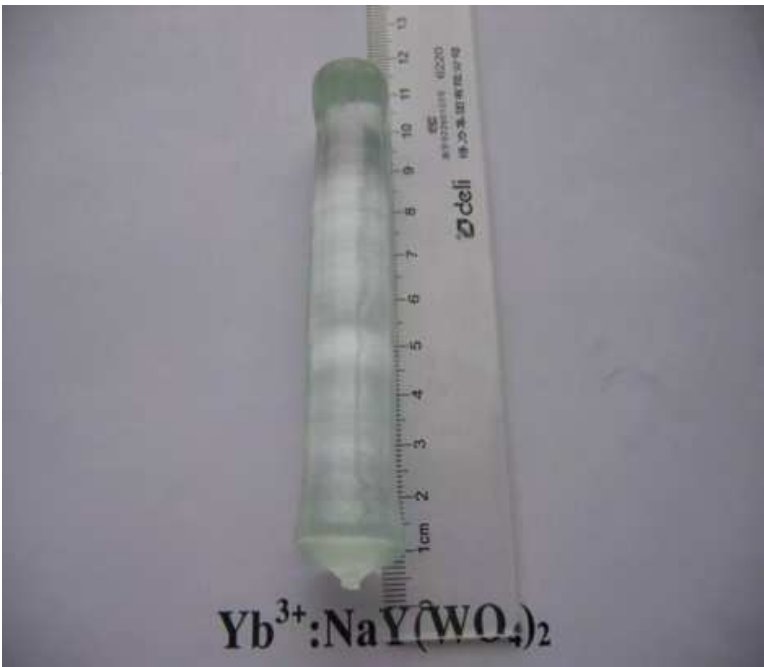
Fig. 2.3 The grown Yb 3+ :NaY(WO 4 ) 2 crystal.
