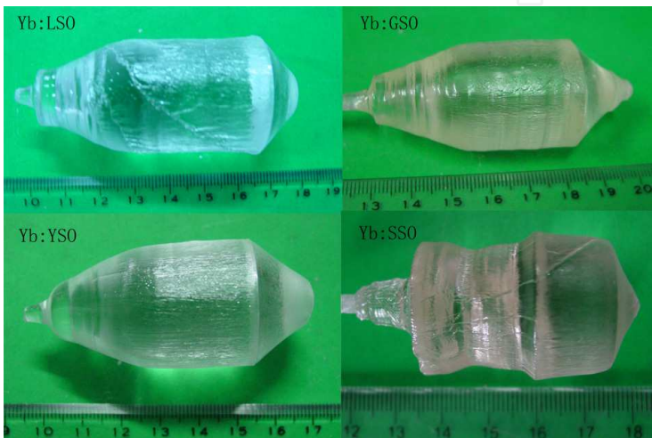
Fig. 1. Bulk crystals of 5at.% Yb doped silicate crystals obtained by Czochralski method.
