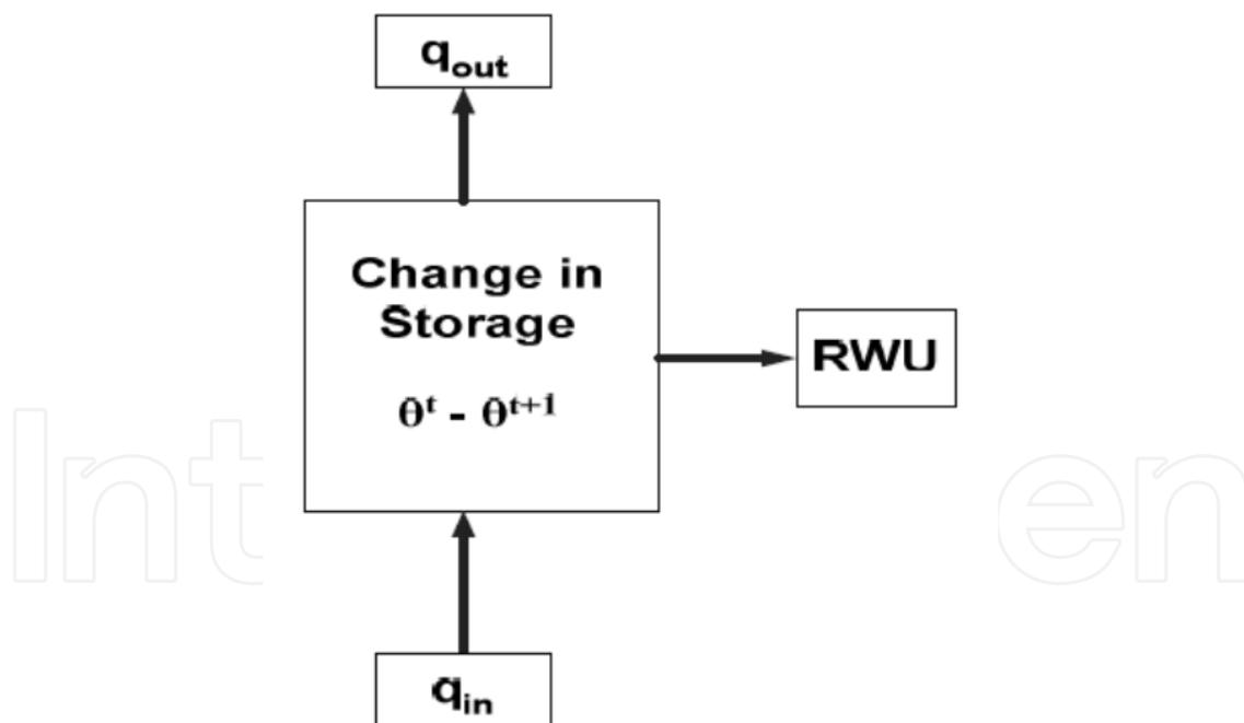
Fig. 9. Schematics of a section of vertical soil column showing fluxes and change in storage.
