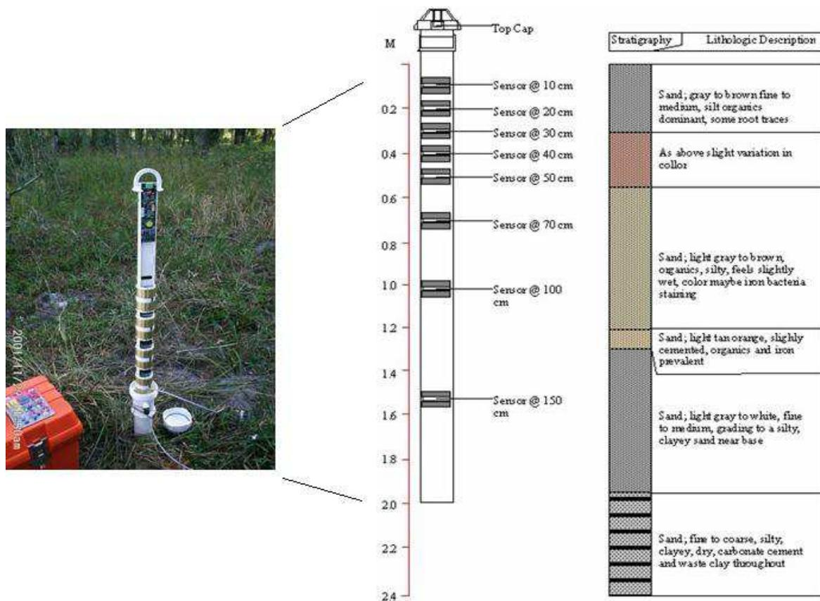
Fig. 2. Soil moisture probe on the left showing the mounted sensors along with schematics on the right showing sample stratigraphy at different depths.
