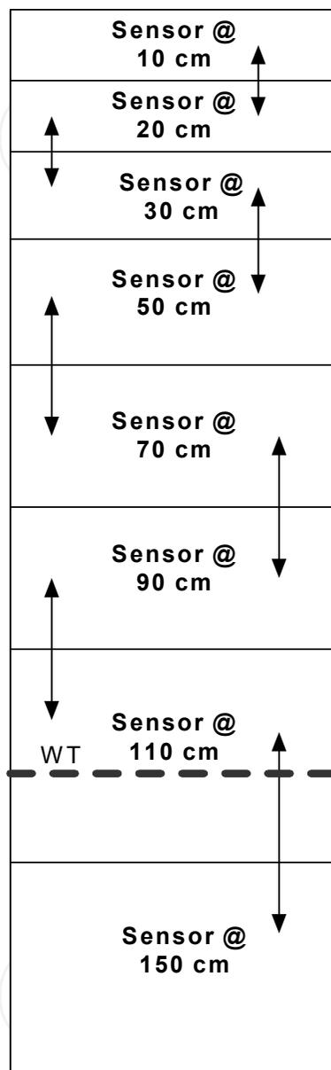
Fig. 8. Schematics of the vertical soil column with location of the soil moisture sensors and water table.
