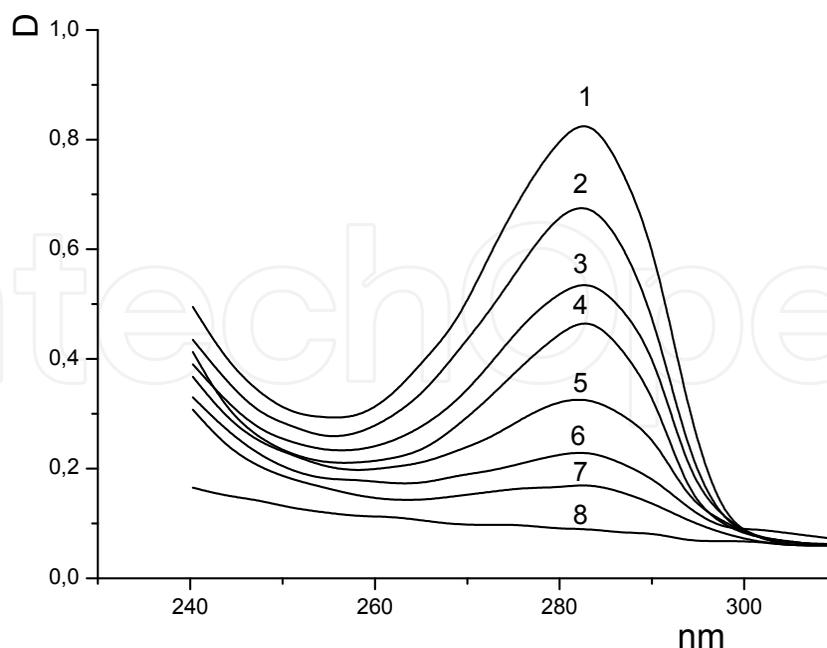
Fig. 4. Change of the DCPA electronic spectrum during irradiation. (1) Starting solution:  $5 \cdot 10^{-4}$  M DCPA; (2–8), solution after UV irradiation for 6, 11, 13, 18.5, 23, 24, and 38 h, respectively.
